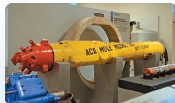
Drilling machine for ducting
